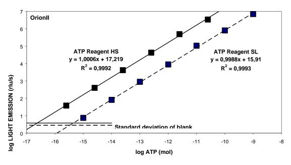
Detection Limit for ATP with ATP Reagent SL: 402 amol/well ATP Reagent HS: 68 amol/well
