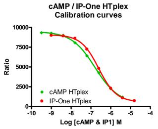
Figure 5. cAMP (green diamonds) and IP1 (red dots) calibration curves.
