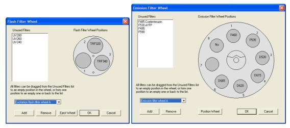
Figure 4a. Instrument settings for HTplex<sup>TM</sup>. Global definition of the optimum excitation filter *TRF340* for Tb cryptates and the emission filters *D520*, *D620* and *D665* for the specific emission spectra of donor and acceptors.
