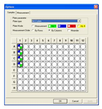
**Figure 3A**: Selection of wells for injections with substrate and treatment. The 4 injectors allow more than one treatment to be added to different wells as desired.
